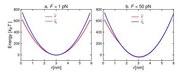
Fig. S1. Comparison of the potentials  $\tilde{V}(r)$  and  $\tilde{V}_s(r)$  at two different forces: (A) F=1 pN; (B) F=50 pN. The energy scales are aligned such that the minima of both potentials occur at 0  $k_BT$ . The parameters are  $k_0=147.2$   $k_BT/nm^2$ ,  $k_1=15.6$   $k_BT/nm^2$ , and  $r_0=3.0$  nm.
