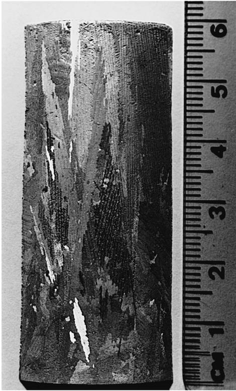
Fig. 4. A chemically etched, exterior slice of a 3 wt.% Sn–Zn ingot directionally solidified at 1.5°C/min. The dendrites that comprise the columnar crystals can be seen because of solidification shrinkage. Compare with Fig. 1.
