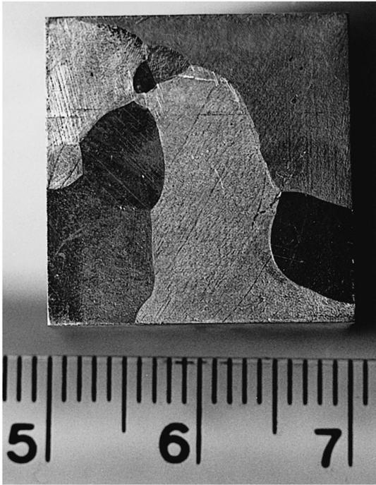
Fig. 6. A chemically etched transverse section of a cube cut from the top of a 100% Zn ingot.
