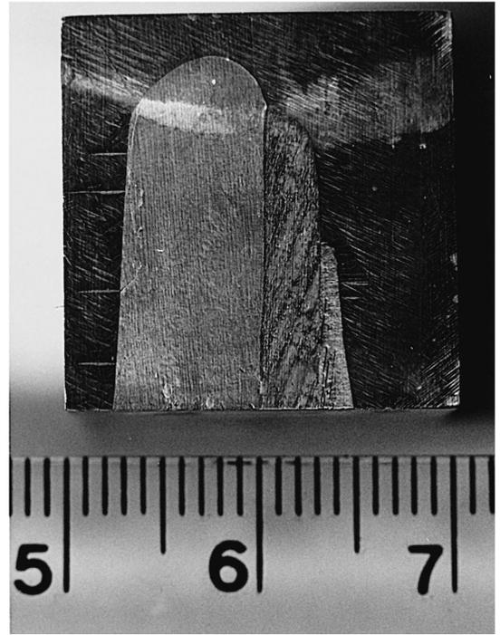
Fig. 7. A chemically etched longitudinal section of a cube cut from the top of a 100% Zn ingot, showing the columnar grains.
