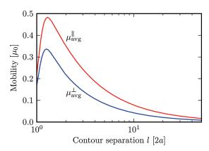
**Figure 4.** Preaveraged mobilities  $\mu_{\text{avg}}^{\parallel}(l)$  and  $\mu_{\text{avg}}^{\perp}(l)$  as a function of contour separation l for a chain with L=100a,  $l_p=20a$ , and F=1.0  $k_BT/a$ .
