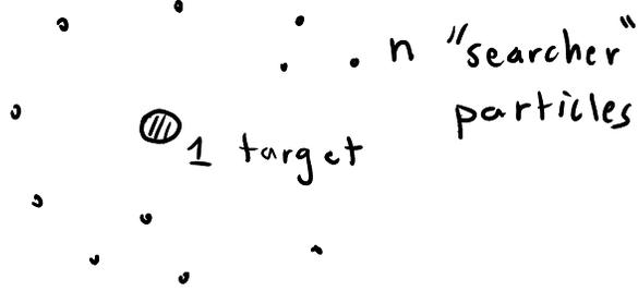
$$\tau = \left( \frac{R_{\max}^2}{6D} \right) \left( \frac{2R_{\max}}{Rn} \right)$$
