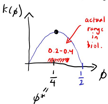
$$\begin{aligned} \frac{dk}{d\phi} &= 0 \\ \Rightarrow \phi &= \frac{1}{4} \end{aligned}$$
